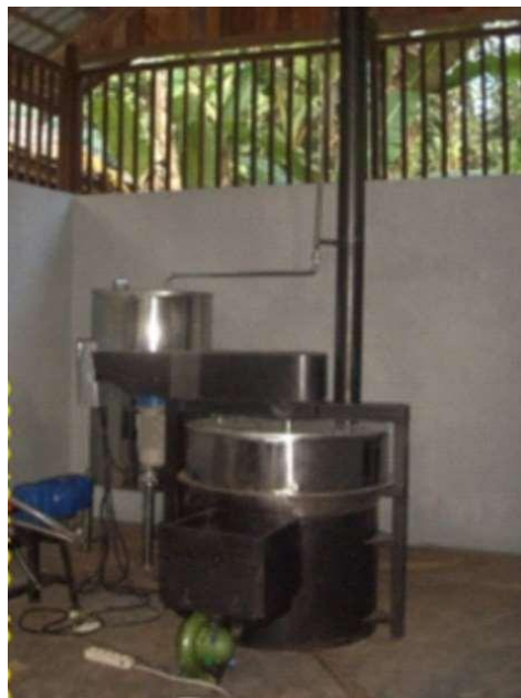
Gambar 2. Mesin Pengolah Gula Aren Modern
